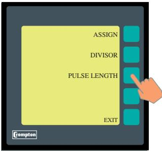
The “PULSE LENGTH” screen enables the width of each output pulse to be adjusted in 20mS increments between 20 and 200mS.
