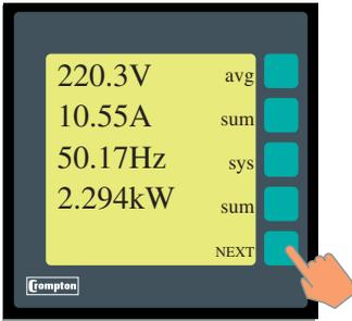
The standard viewing screen has four active readings indicated.
