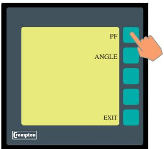
On pressing **"PF PA"** the display offers two choices for displaying the phase relationships: Power Factor (**"PF"**) and Phase Angle (**"ANGLE"**).
