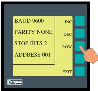
This screen allows the user to configure the parameters for the RS485 port. *NOTE: Communicatios settings for Johnsons Controls are fixed and pre set.* A pointer is shown next to the value being changed. The "INC" and "DEC" keys are used to increment and decrement the displayed value. The "ROW" key is user to move the pointer to the next parameter.
