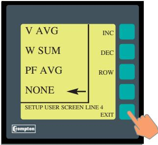
If any line is assigned to be "NONE", a blank space will be shown. If all four lines are assigned "NONE" the factory default screen of Vavg, Asum, Hz and Wsum is shown.
