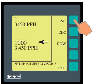
NOTE: If the system power is scaled in kW then the default pulse rate is 1 pulser per kWh (up to 3,600 kW system). If the system power (see system settings) is over 3.6 MW then the pulse rates adjust accordingly to 1 pulse per MWh.
