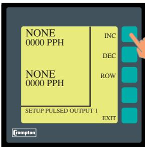
This screen assigns a parameter to each of the pulsed outputs.
