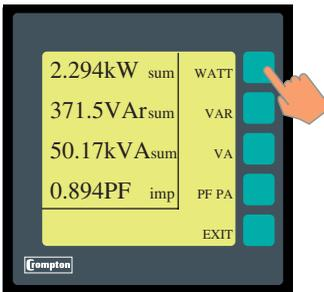
The first level power screen by default shows active readings of W, VAR, VA and PF PA.
