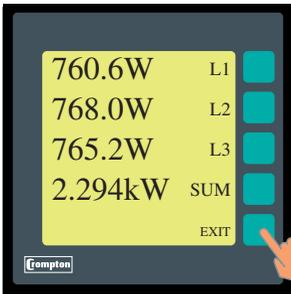
This will expand the active screen to full size. This screen remains until deactivated by pressing **"EXIT"** where it will return to the reduced active screen.
