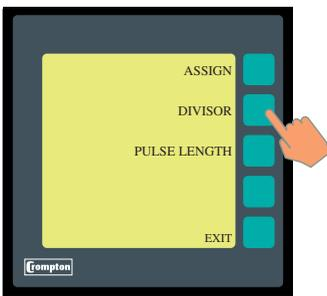
The "DIVISOR" screen enables a divide ratio of 10, 100 or 1000. This allows the user to program the unit to output a lower number of pulses according to the system requirements. For example, setting the divisor to 1000 will output kilowatt hour pulses, and setting the divisor to 1 will output Watt hour pulses.
