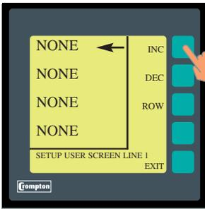
This screen assigns a parameter to each of the four screen lines.
