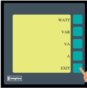
Press **"WATT"** to zero accumulated W.h. **"RESET"** will appear to the left indicating this choice has been made. A similar function is performed by the **"VAR"**, **"VA"** and **"A"** keys.
