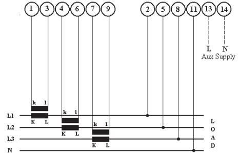
**Wiring** - Input connections are made directly to shrouded screw clamp terminal. Numbering is clearly marked on the plastic moulding. Choice of cable should meet local regulations. Terminals for both current and voltage inputs will accept up to 3mm<sup>2</sup> x 2 diameter cables.
